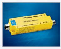
TURCK'S new interface module cartridge (IMC) series is another innovative breakthrough in process automation: The I.S. barrier is moved from the mounting cabinet directly to the installation, thus making it possible to create further decentralized structures in the installation.
