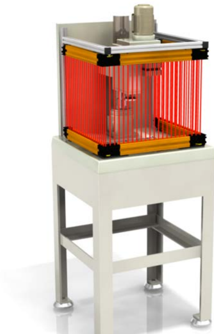
Figure 43. Cascaded light screens guarding a u-shaped cell
