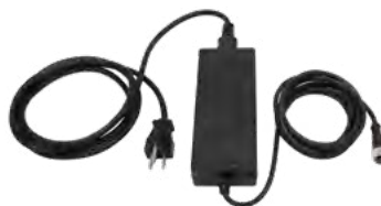
PSD-24-4 Class 2 Power Supply Input: 90-264 V ac 1.5A Output: 24 V dc 3.9A 2 m 4-Pin Euro
