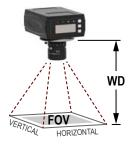
Figure 394. Working Distance and Field of View
