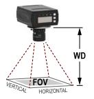
Figure 397. Working Distance and Field of View
