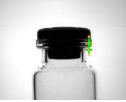
Figure 215. Edge Tool at the Right Side of the vial
