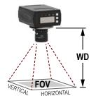
Figure 396. Working Distance and Field of View
