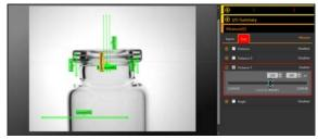
Figure 220. Bad Part-Missing Stopper
