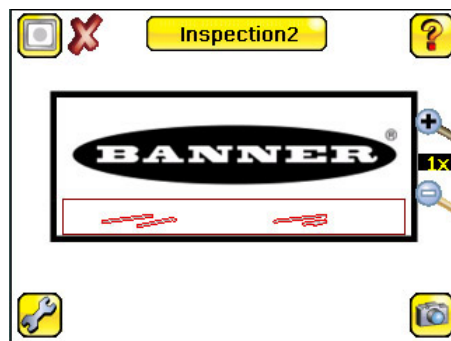
Figure 111. Blemishes Found During the Inspection
