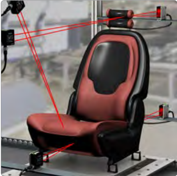
Auto seat adjustment measurement using the LE550
