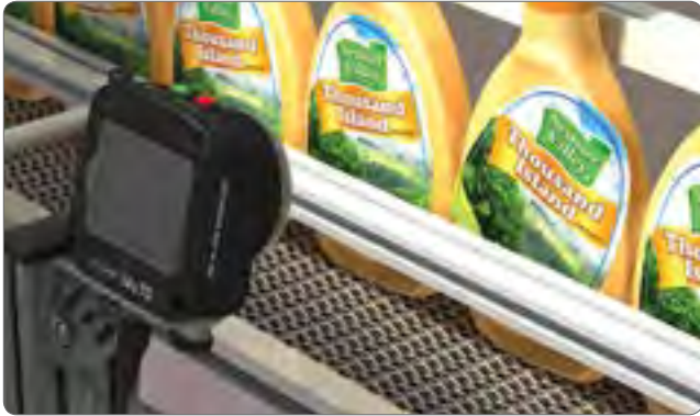
Label detection using a Match Sensor
