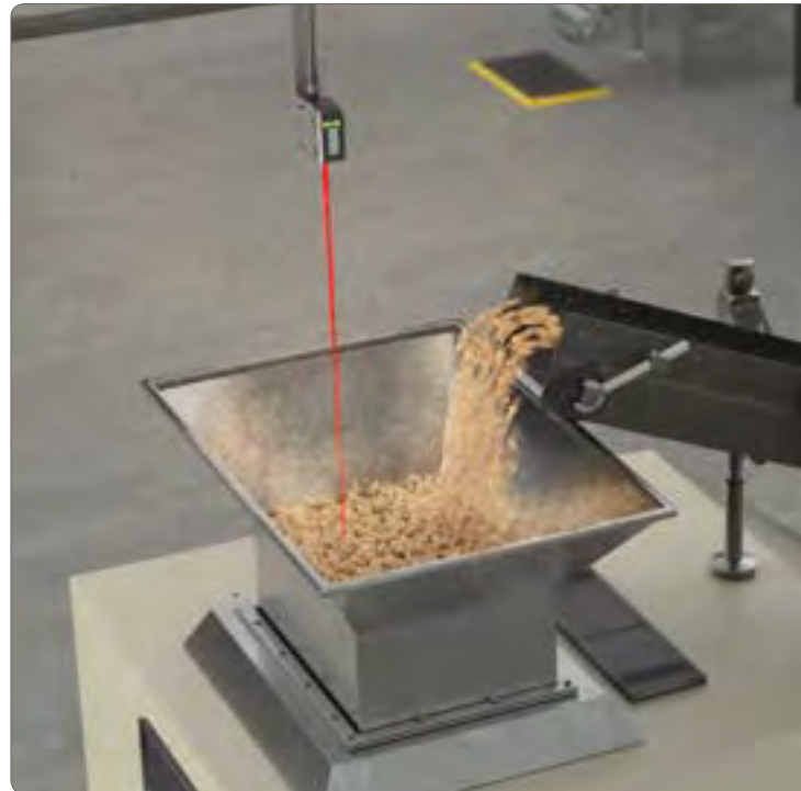
Monitoring levels inside a high-volume hopper
