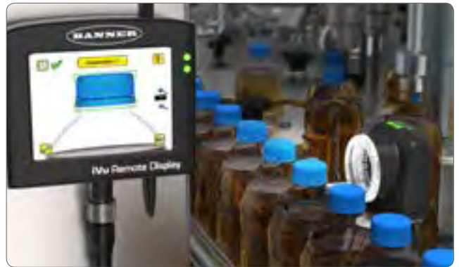
Cap verification using a Color Area Sensor
