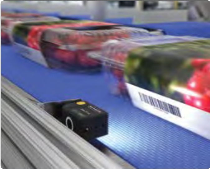
Barcode reading for food traceability
