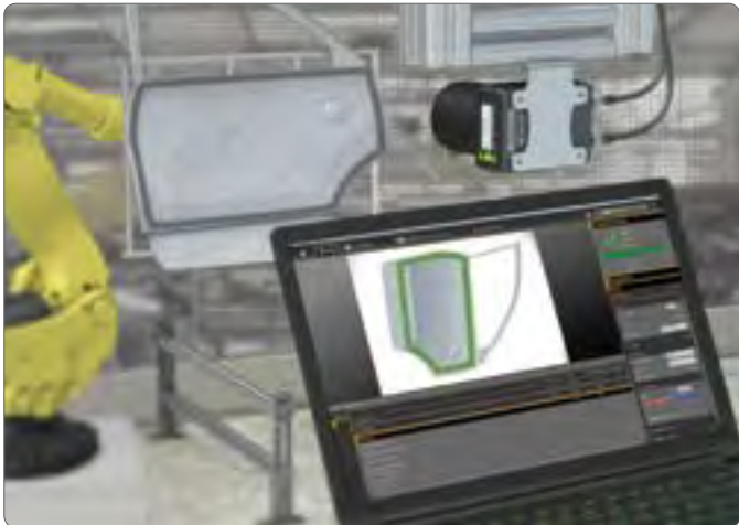
Door panel adhesive inspection using Bead Tool
