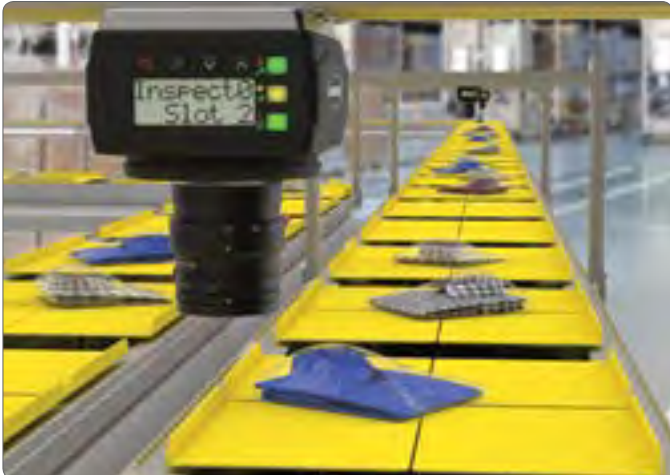
Empty sortation conveyor inspection using Blemish Tool
