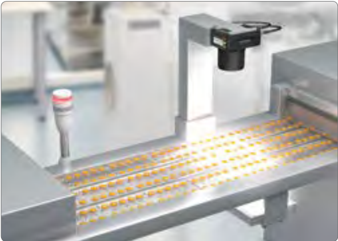
Blister pack inspection using BLOB Tool
