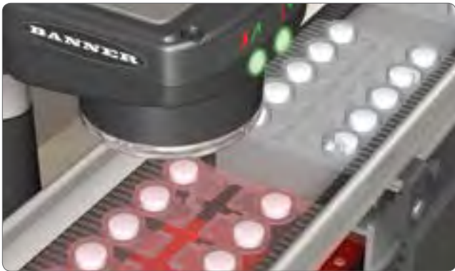
Blister pack inspection using an Area Sensor
