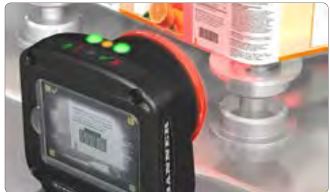
Label verification on labeler machine
