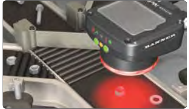
Hardware sortation using a Sort Sensor
