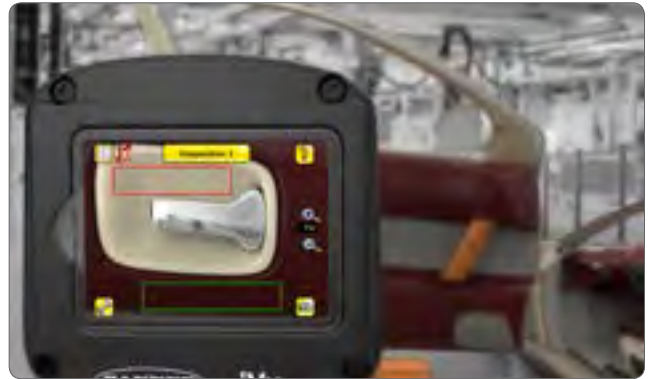
Trim color verification using an Average Color Sensor
