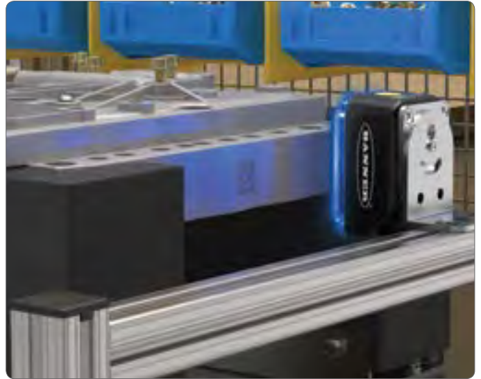
Direct Part Mark (DPM) code reading and verification on automotive part
